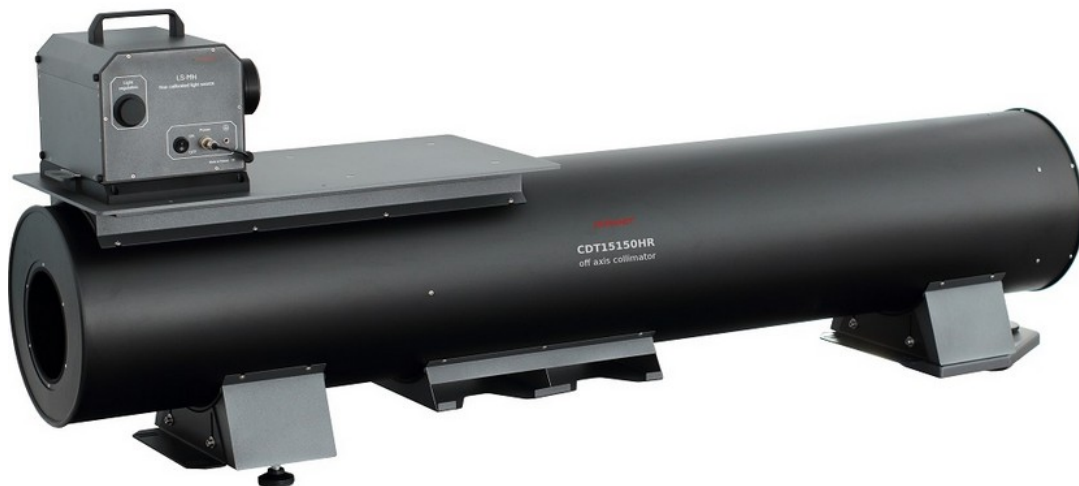
Fig. 1. LS-MAH light source as a part of VINIS test system for testing VIS-NIR cameras
